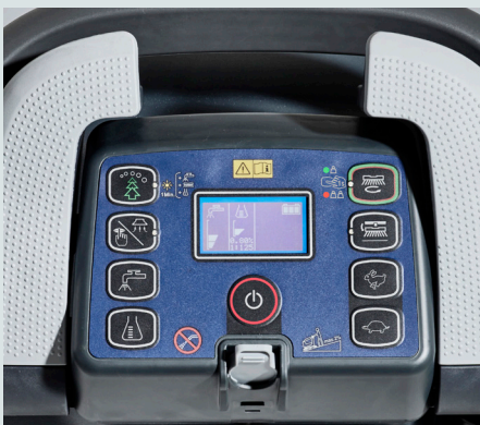
Informative digital display, intuitive icon buttons and new ergonomic drive paddle
