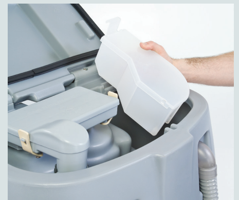
A debris tray captures the dirt from the suction hose to prevent it from entering the recovery tank
